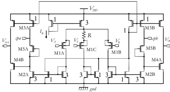
Figure 3: TIA complete schematic diagram.
