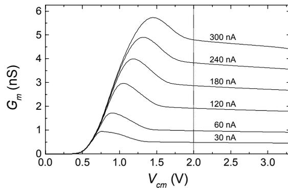
Figure 6:  $G_m$  plots as a function of the input common mode voltage for various tuning current values.
