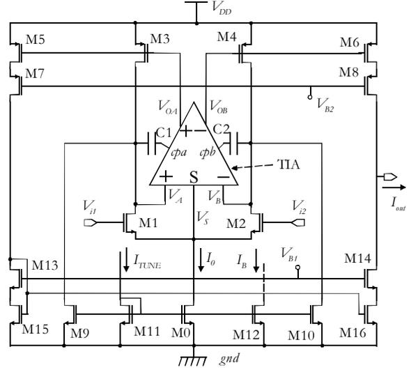
Figure 2: Complete schematic diagram of proposed transconductor.  $I_B$  provide biasing of the TIA block;  $V_{B2}$  and  $V_{B1}$  are bias voltages for the M5-8 and M9-16 cascode mirrors, respectively.
