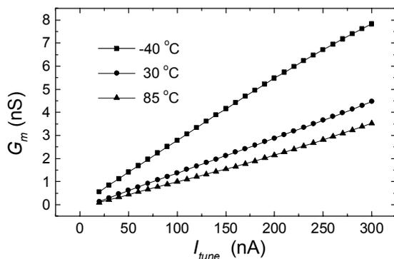
Figure 5: Tuning law for three different temperatures.
