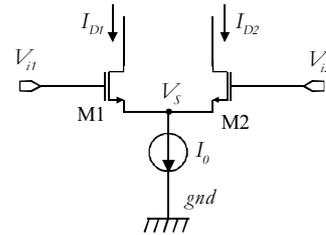
Figure 1: Basic source coupled pair
