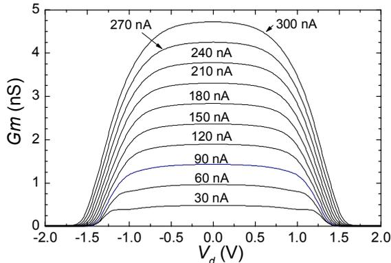
Figure 4:  $G_m$  vs.  $v_d$  for various tuning currents.
